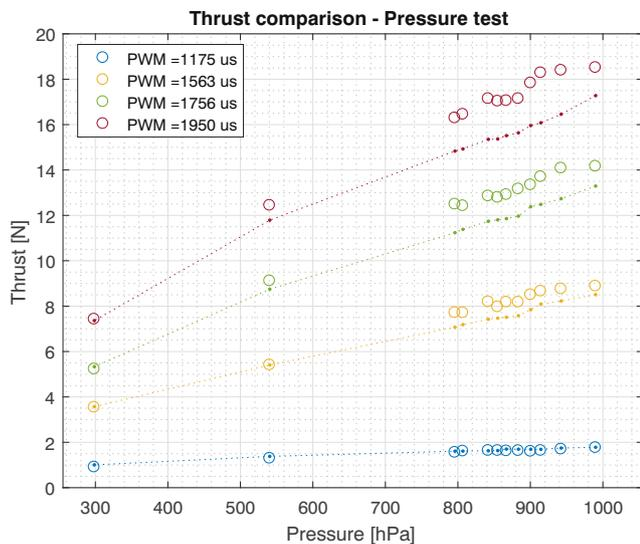
**Fig. 22** Propeller thrust comparison between experimental data collected inside terraXcube and Blade Element Theory for pressure test. The dotted curves are the values computed using BET while the circle markers are the measurements of the tests
