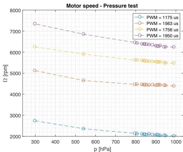
Fig. 14 Measured motor speed for pressure tests
