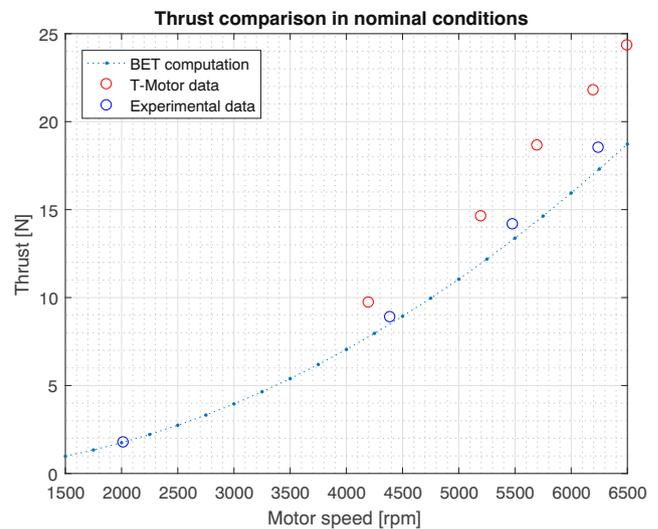
Fig. 20 Propeller thrust comparison between Blade Element Theory, T-Motor [5] and measurements collected inside terraXcube at 990 hPa and 30.2°C
