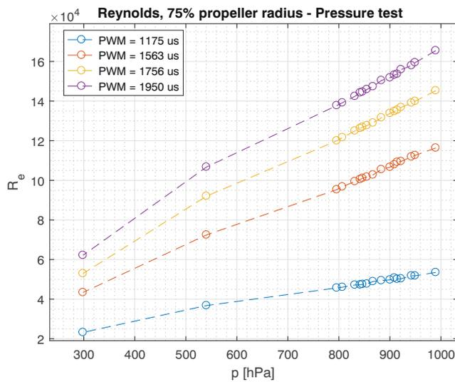
Fig. 18 Reynolds number computed at 75% of the propeller radius for pressure tests
