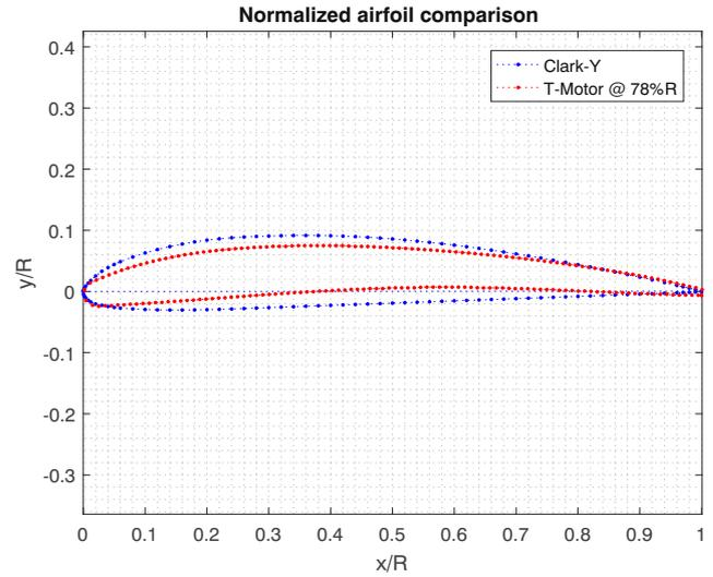
Fig. 19 Comparison between T-Motor profile at 75% of the propeller radius and Clark-Y airfoil
