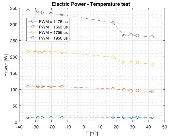
Fig. 7 Electric power for temperature tests
