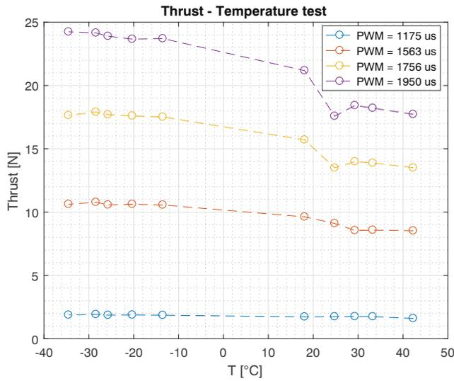
Fig. 5 Measured propeller thrust for temperature tests
