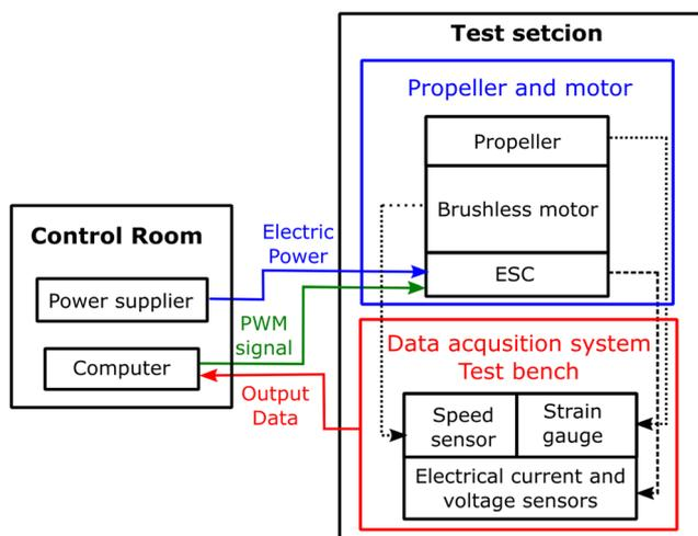
**Fig. 4** Schematic of the data acquisition, control and power system for the tests
