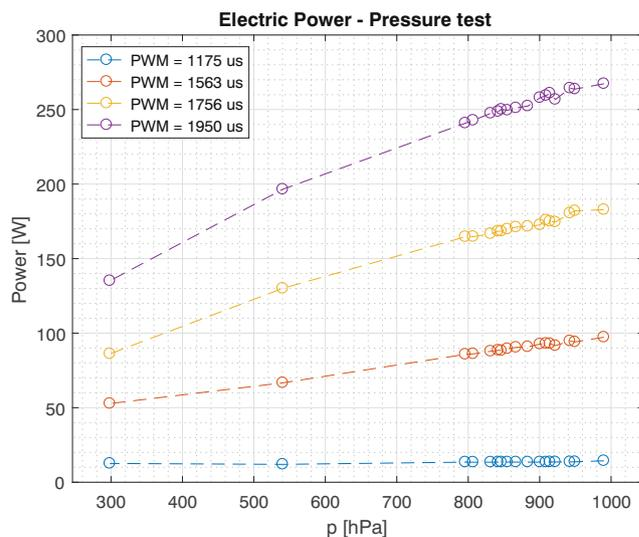
Fig. 15 Measured electric power for pressure tests. Electric current reveals a similar behaviour
