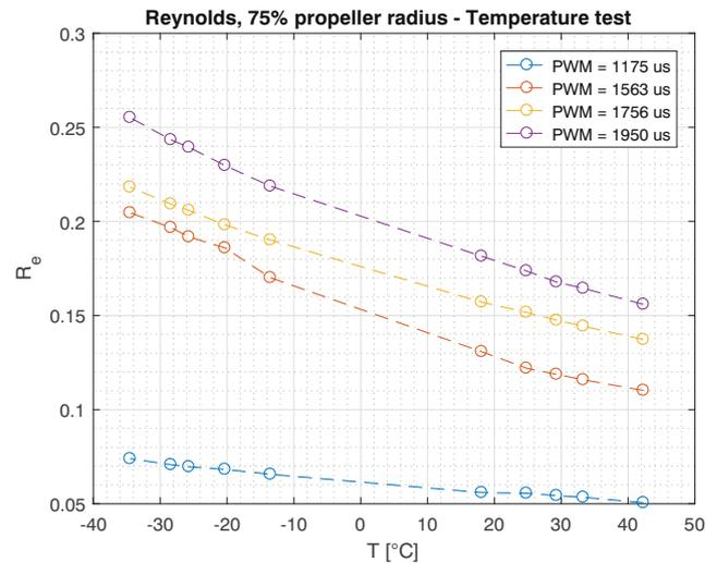
Fig. 12 Reynolds number evaluated at 75% for temperature tests
