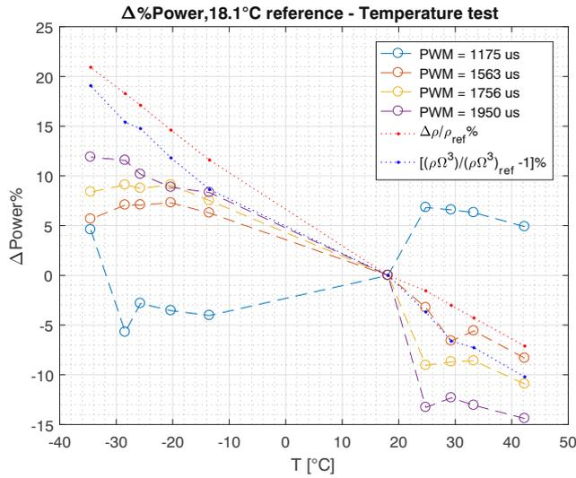
Fig. 9 Computed percentage change of electric power for temperature tests
