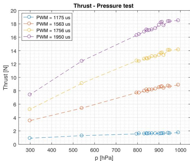
Fig. 13 Measured propeller thrust for pressure tests
