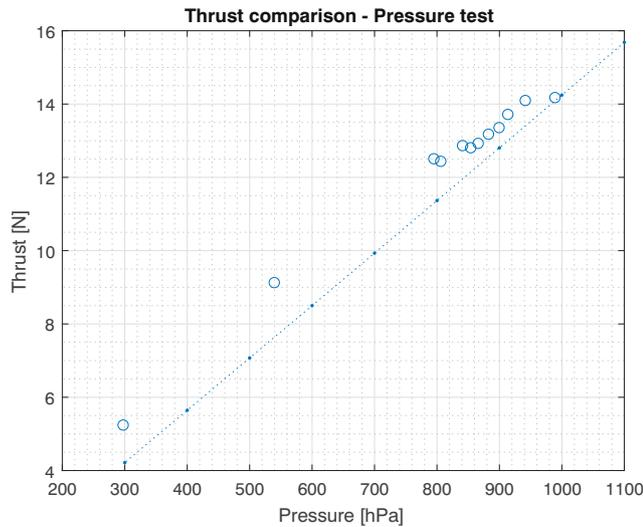
**Fig. 24** Thrust computed at constant motor speed for pressure tests. Circles are the experimental data measured at constant PWM
