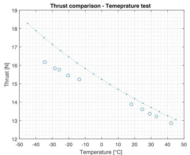
**Fig. 23** Thrust computed at constant motor speed for temperature tests. Circles are the experimental data measured at constant PWM
