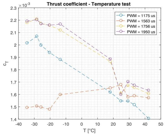
Fig. 11 Propeller thrust coefficient for temperature tests
