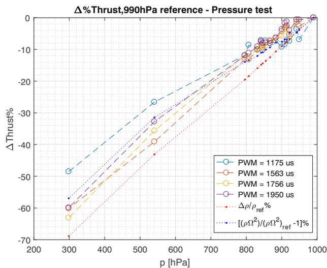
Fig. 16 Computed propeller thrust percentage change for pressure tests. Electric power experience the same trend
