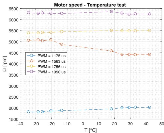
Fig. 6 Measured motor speed for temperature tests
