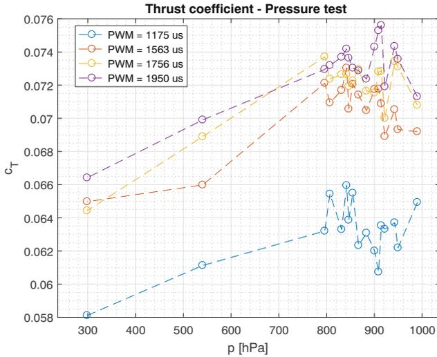
Fig. 17 Computed thrust coefficient for pressure tests
