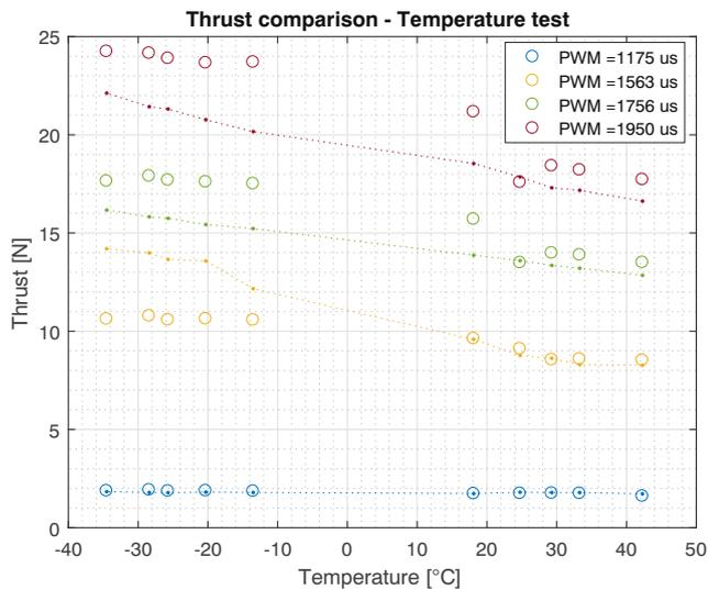
**Fig. 21** Propeller thrust comparison between experimental data collected inside terraXcube and Blade Element Theory for temperature test. The dotted curves are the values computed using BET while the circle markers are the measurements of the tests
