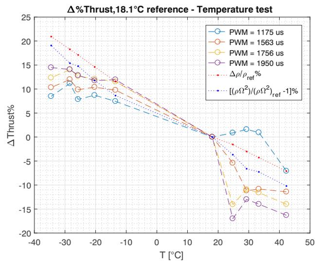
Fig. 8 Computed percentage change of propeller thrust for temperature tests
