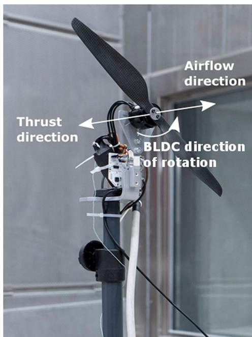
**Fig. 2** Rotor assembly and schematic of thrust and airflow directions
