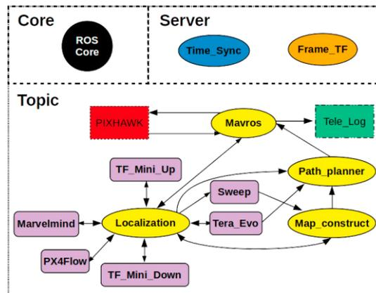
Fig 3. ROS diagram on Raspberry Pi 3B+
