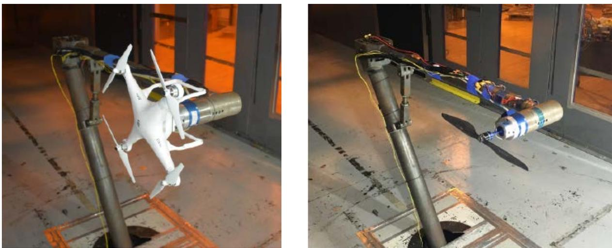
Figure 4: NASA Ames Multicopter Wind Tunnel Test. Photographs taken from [10]
